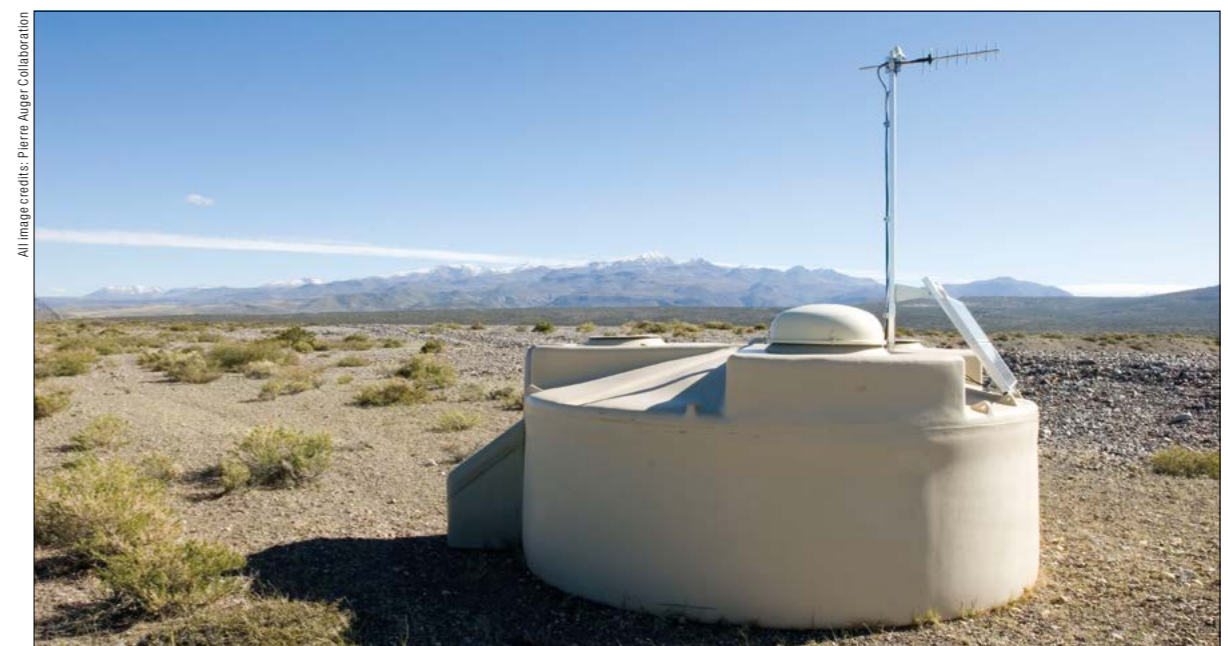
An Auger Observatory water-Cherenkov surface detector on the Pampa Amarilla.
