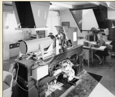
ERASME, the latest scanning and measuring system at CERN. It combines both stages and allows operator intervention in the measurement process to an extent that has not been possible before. ERASME is designed to handle film from the Big European Bubble Chamber (BEBC).
