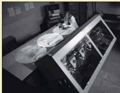
A SAAB scanning table, designed to cope with the special film from the heavy liquid bubble chamber, Gargamelle. The chamber volume is covered by separate cameras and separate images can be projected. Measurement is carried out online with a computer.
