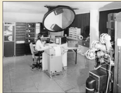
An LSD (or Spiral Reader) measuring machine, which receives film previously scanned on Shivamatic scanning tables. An operator is involved in the measurement process to set the machine on the vertex of the event to be measured. A slit, moving in a spiral, then searches the film and sends track information to a computer.
