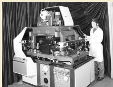
An HPD, which carries out precise measurement, automatically without human intervention, on the film previously scanned on a MILADY table. An optical-mechanical spot sweeps over the film and full track co-ordinates are transmitted to a computer.
