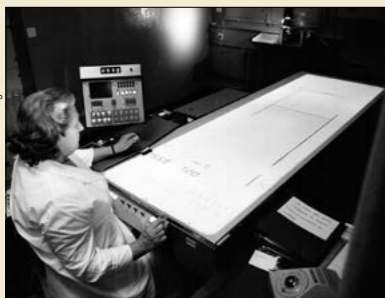
Studying bubble-chamber film on one of the MILADY scanning tables, where sufficient information is collected to be able to tell the Hough-Powell Device (HPD) measuring machines where to look. The operator picks out events of interest on the film and records details such as vertex position and a few track co-ordinates on magnetic tape.
